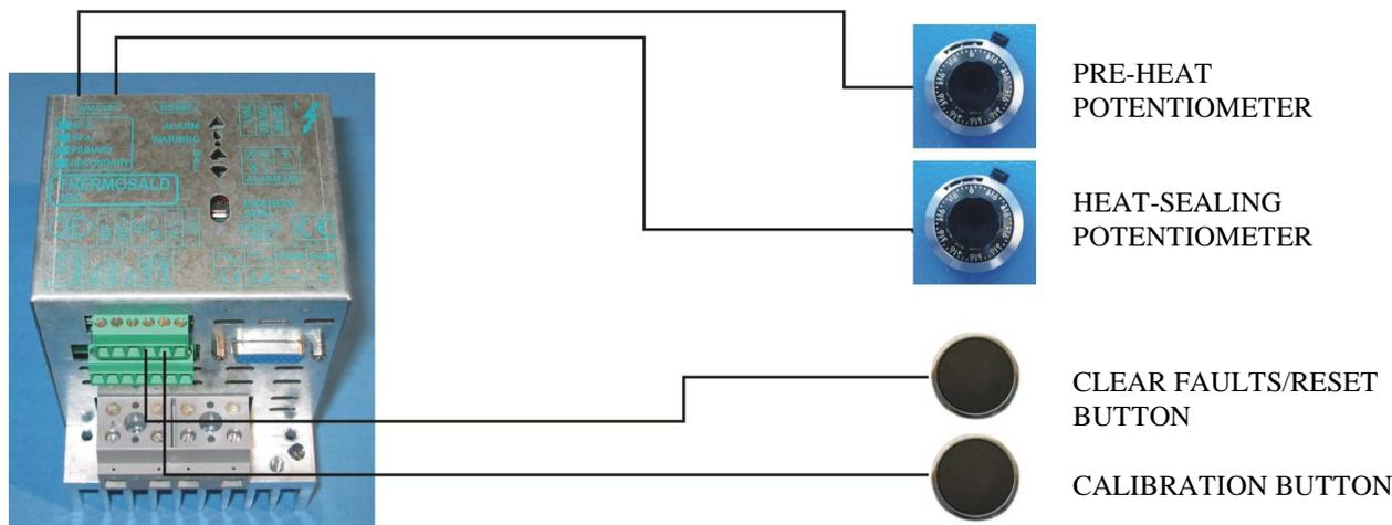
**Step 1** – Calibrate the system after performing the steps indicated in paragraph 4.1.
