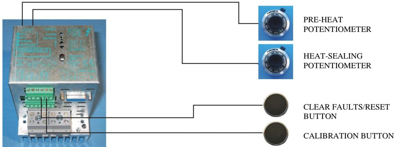
**Step 1 – Calibrate the system after performing the steps indicated in paragraph 4.1.**
