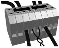
Power terminals must have screws so an optimal connection is guaranteed (do not use terminals with springs or similar) and must be positioned as near as possible to the sealing bars.
