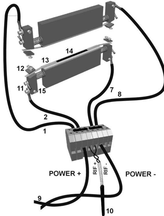
The previous picture shows a wiring with two bands in parallel (cables 1,2,7,8): for one single band use only two cables (e.g. 1,8).
