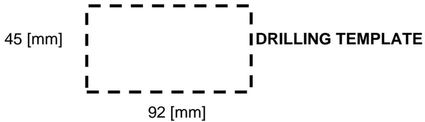
**NOTE:** with IP65 protection, code 3ES108Z=IP65, the drilling template must be 94mm x 47mm. The maximum outside dimension is 102mm x 54mm.
