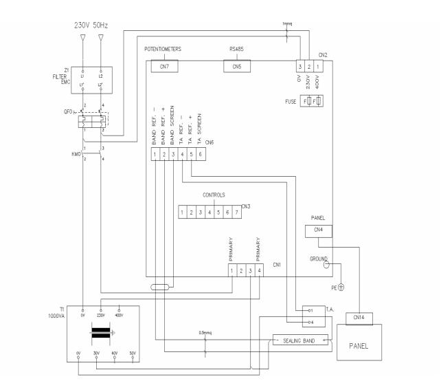
NOTE -Power supply (CN1/1 e CN1/4) must be with the same phase as control supply (CN2/3 e CN2/2). Ground screw must be connected to the ground of machine, with the cable jellow green section > = power cable section. Twist power cable, twist TA cable Twist and screen sealing reference cable
