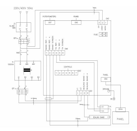
NOTE -Power supply (CN1/1 e CN1/2) must be with the same phase as control supply (CN2/3 e CN2/2). Ground screw must be connected to the ground of machine, with the cable jellow green section > = power cable section. Twist power cable, twist TA cable Twist and screen sealing reference cable
