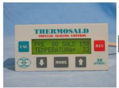
NOTe: To scroll the sub-menus, press buttons MODE+ARROW DOWN or ARROW UP in the order given.
