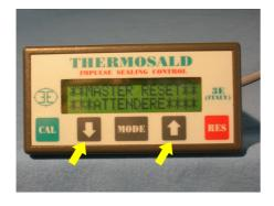
Using the Master Reset procedure the thermoregulator self-configures according to the hardware installed. The parameters are initialized as factory set: if a parameter has been changed, it must be returned to the working condition.
