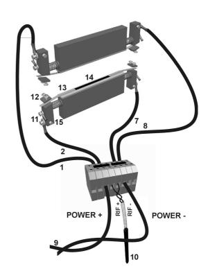
Warning: one end of the band's power circuit is connected to PE; this connection is made in the grey power terminal block CN1, terminals 2 and 3. Do not ground the band directly.
