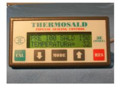
To perform a **MASTER RESET** keep the arrow up and arrow down button pressed for 6 seconds until figure 5.4.2 is displayed
