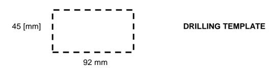
NOTE: with IP65 protection, code 3ES108Z=IP65, do drilling template 94mm x 47mm, Maximum external size 102mm x 54mm
