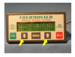
procedure Using the Master Reset thermoregulator self-configures according to the hardware installed. The parameters are initialized as factory set: if a parameter has been changed, it must be returned to the working condition.
