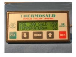
To perform a **MASTER RESET** keep the arrow up and arrow down button pressed for 6 seconds until figure 5.4.2 is displayed
