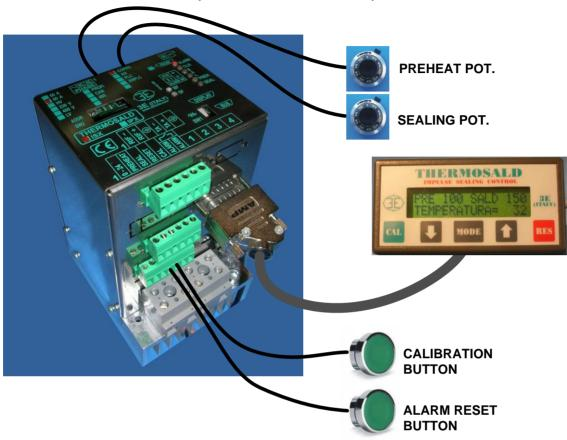
NOTE 1: set the CONFIGURATION MACHINE DATA=1 potentiometers+display to enable the potentiometers.
