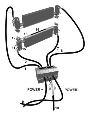
The previous picture shows a wiring with two bands in parallel (cables 1,2,7,8): for one single band use only two cables (e.g. 1,8).
