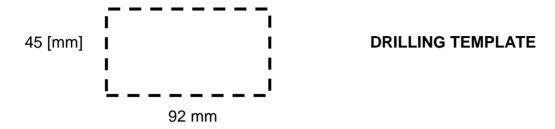
NOTE: with IP65 protection, code 3ES108Z=IP65, do drilling template 94mm x 47mm, Maximum external size 102mm x 54mm
