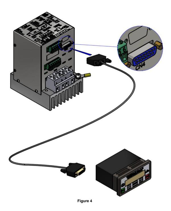
The connection cable between the thermoregulator and the display panel must be shielded with pin-to-pin connection. Cable core section must be at least 0.25 mm<sup>2</sup> and maximum length 20 m. It is advisable to use cables supplied by 3E available in various lengths (see par. 11.1.13).
