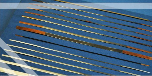
Figure 31 - Coppered, silver-plated and nickel-plated sealing bands
