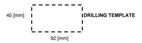
NOTE: with IP65 protection, code 3ES108Z=IP65, the drilling template must be 94mm x 47mm. The maximum outside dimension is 102mm x 54mm.
