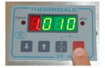
On the display appears "H100", to inform that the first heating at 100 degree is in progress; next the writing H200, H100, H200, H100, H200, H100 will appear to inform that cycles of heating and colding at 200 and 100 degrees are in progress. At the end the termoregulator will be ready to work. Burn in cycle can be stopped before end pressing key reset.
