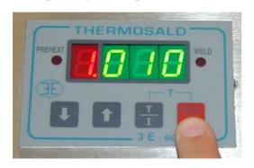
On the display appears " H100", to inform that the first heating at 100 degree is in progress; next the writing H160, H100, H160, H100, H160, H100 will appear to inform that cycles of heating and colding at 160 and 100 degrees are in progress. At the end the termoregulator will be ready to work.
