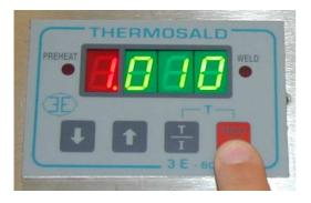
On the display appears "H100", to inform that the first heating at 100 degree is in progress; next the writing H200, H100, H200, H100, H200, H100 will appear to inform that cycles of heating and colding at 200 and 100 degrees are in progress. At the end the termoregulator will be ready to work.
